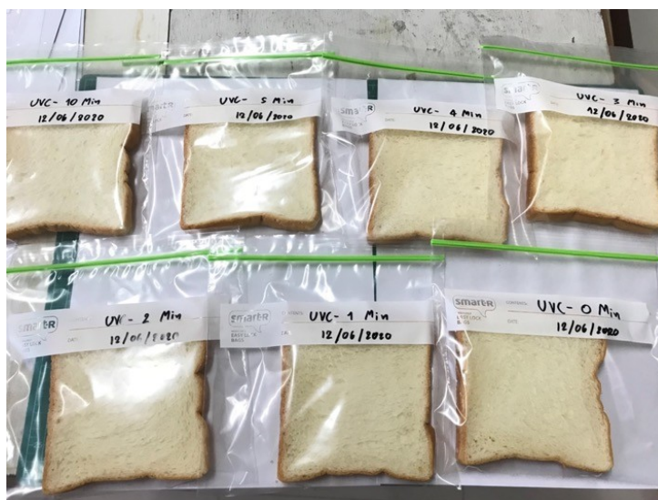
Figure 5. Breads in Ziplock Bags Prepared for UV-C Exposure at Different Durations Ranging from 0-5 and 10 Minutes
